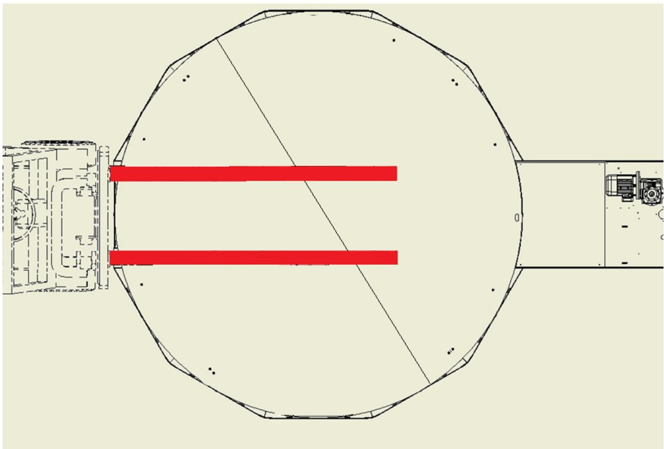
7) Screw the plates on the frame to realize the surface and to allow the passage of the transpallet.
