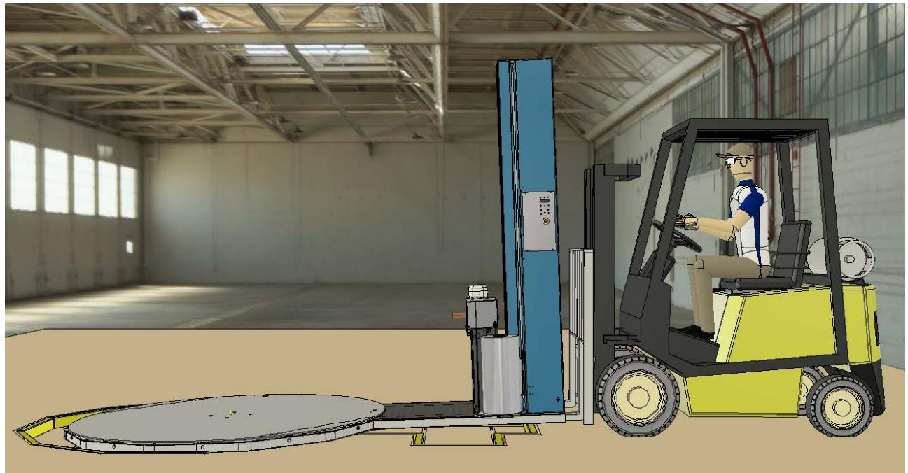
If the turntable of the machine is larger than 2400 of diameters, the operator has to put the fork lift truck on the front side of the turntable as show in picture below.
